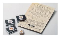
Certified standards for calibrating the SIG-MASCOPE® SMP10 are traceable to internationally recognized calibration standards.
