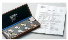
Internationally recognized Boeing Standards are used to establish the working standards of the SIGMASCOPE® SMP10.
