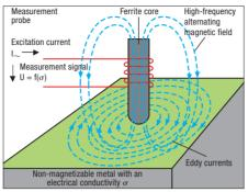
The eddy currents generated by the magnetic field of the probe and utilized as the measurement effect are influenced by the electrical conductivity.
