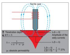
The penetration depth  $\delta$  of the eddy currents is established by the measurement frequency f, which determines the minimum permissible thickness of the specimen.
